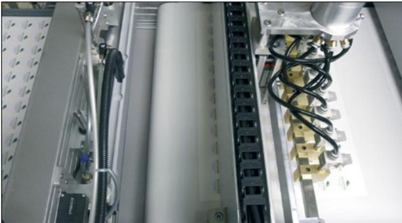
*The prefabricated sheets are guided automatically to the conveyor belt. They are laid on the belt, the system puts single-component resin on the stickers, and the belt then transports the sheets into the ultraviolet light tunnel.*
